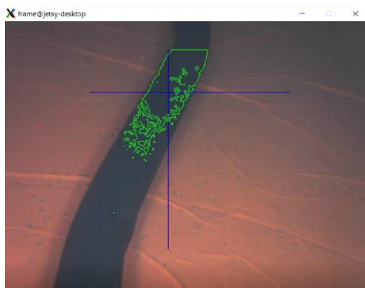
Fig 17. The results of testing the detection program with dark lighting parameters with the help of a 12 V LED light
