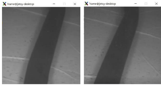
Fig 5. The results of the process of converting RGB to gray format (left) and the results of the blurring process (right)
