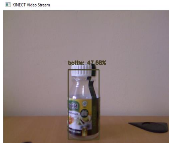
Fig 13. Example of BNU 4.0 Robot object detection results using Deep Learning
