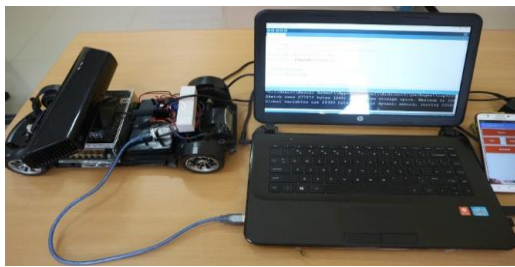
Fig 10. Programming the Arduino Smart Robot BNU 4.0 via a USB connection
